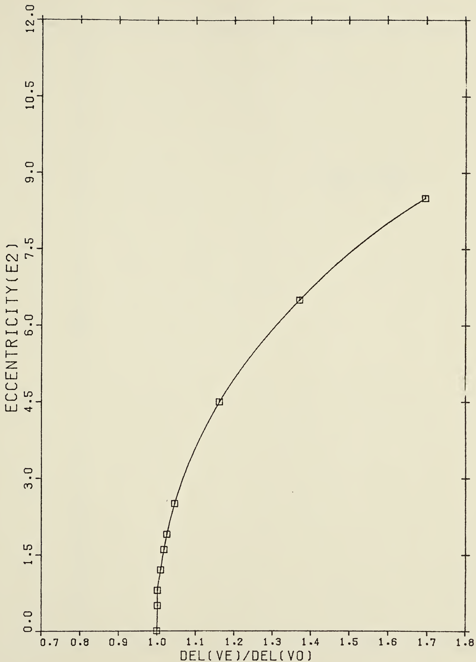
Figure 6.2 Variation of Midspan Deflection With Eccentricity
